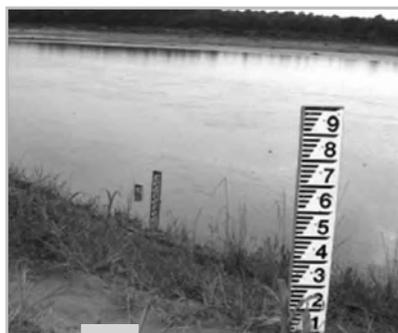
Figure 4.3: Water level-gauge installed at the river bank
